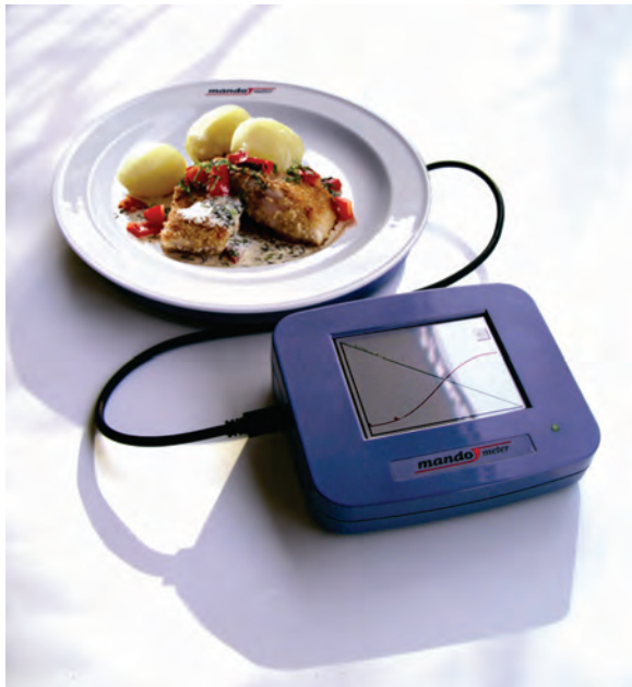
Figure 2. Mandometer ® , a personal computer connected to a scale recording the weight loss of a plate during the meal. Feedback on how to eat can be provided on the touch screen.
